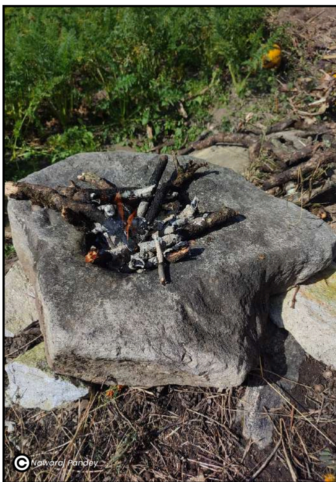
Before oil pressing: Heating the Okhal (stone mortar)
